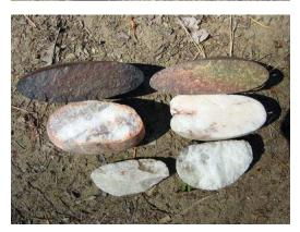
Quartzite fared a little better, being smaller-grained and more homogenous throughout it's structure. About 50% of these survived. I will note that when quartzite cracked, it sometimes exploded (but shards never traveled more than a foot or so away from the wooden bowl. And the winner is...
