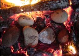
Poor granite. This species suffered a near 100% failure rate. I've been told by a geology professor that water can infiltrate the interstitial spaces between the relatively-large quartz, feldspar and mica crystals and expand the rock when heated. To it's credit, granite never sent shrapnel flying when it cracked.
